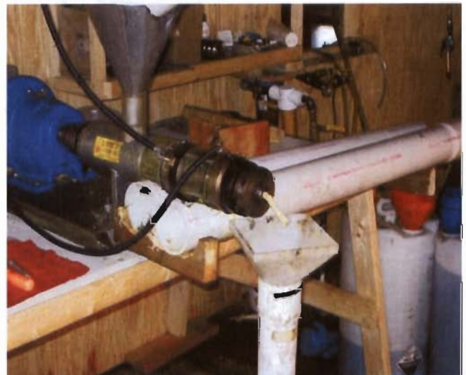
Soybean and sunflower seeds being pressed for oil and meal
